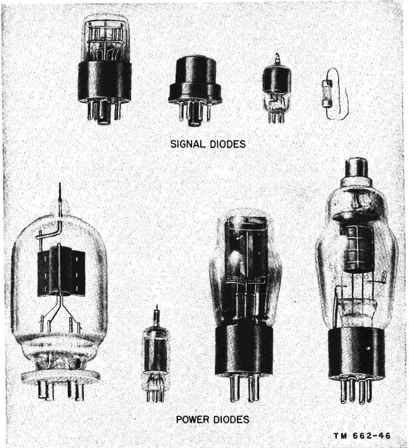
Figure 37. Various types of high-vacuum diodes.
