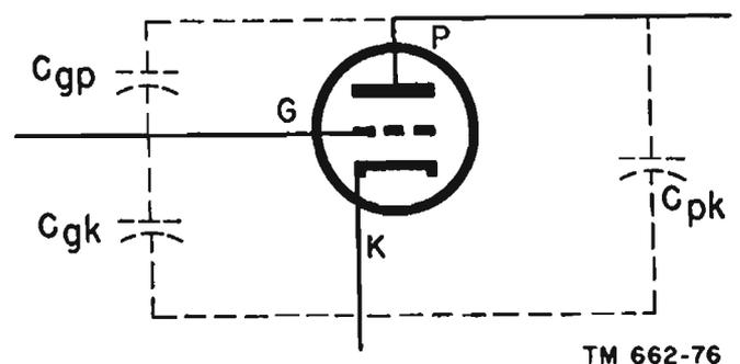
Figure 67. Location of interelectrode capacitances within triode.
