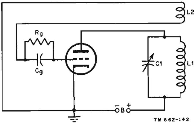
Figure 133. Tuned-plate oscillator.
