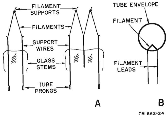
Figure 15. Directly heated filaments and schematic symbol.
