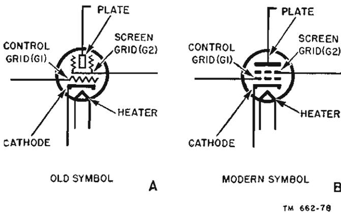
Figure 69. Tube symbols for tetrode.
