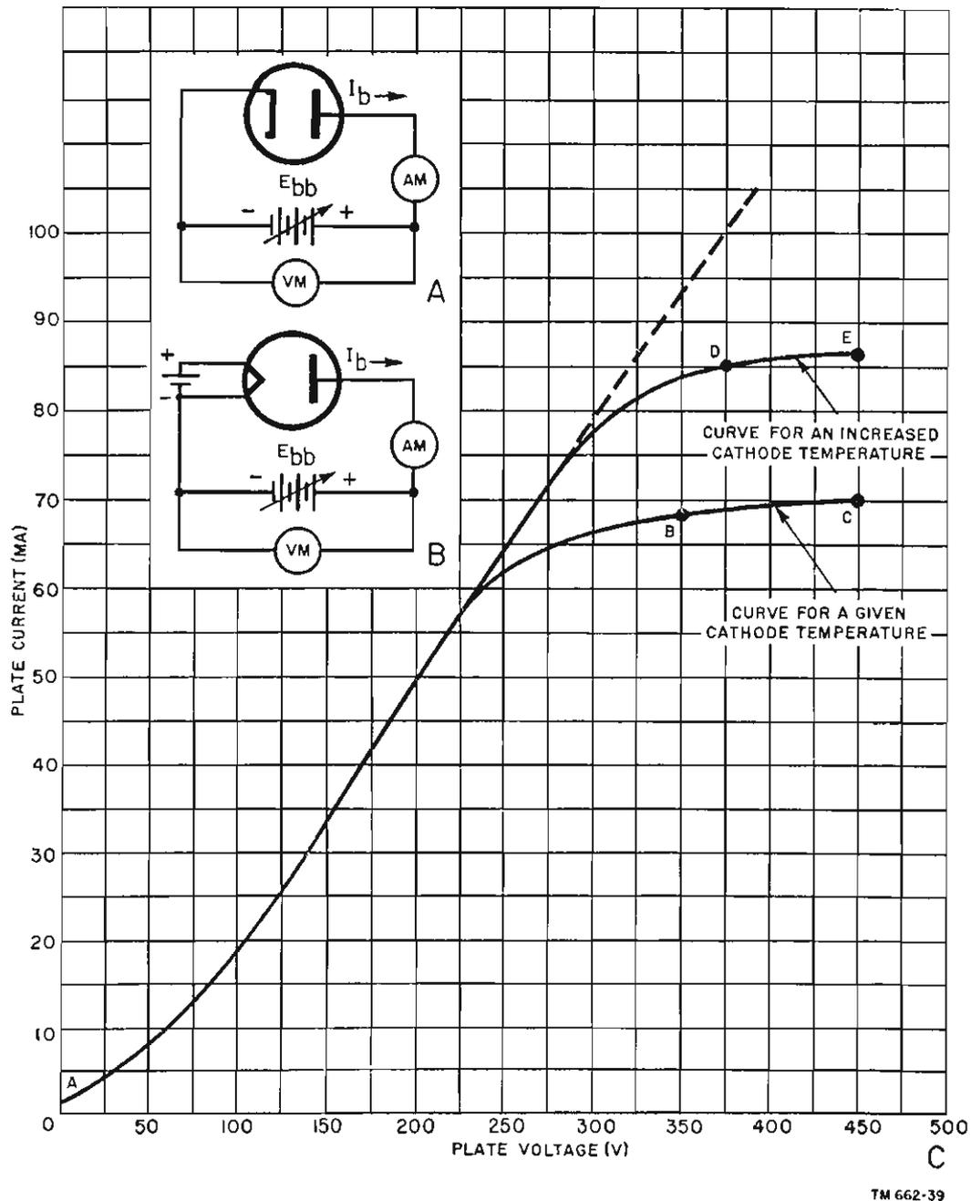
Figure 30. Plate-current plate-voltage characteristic curves.
