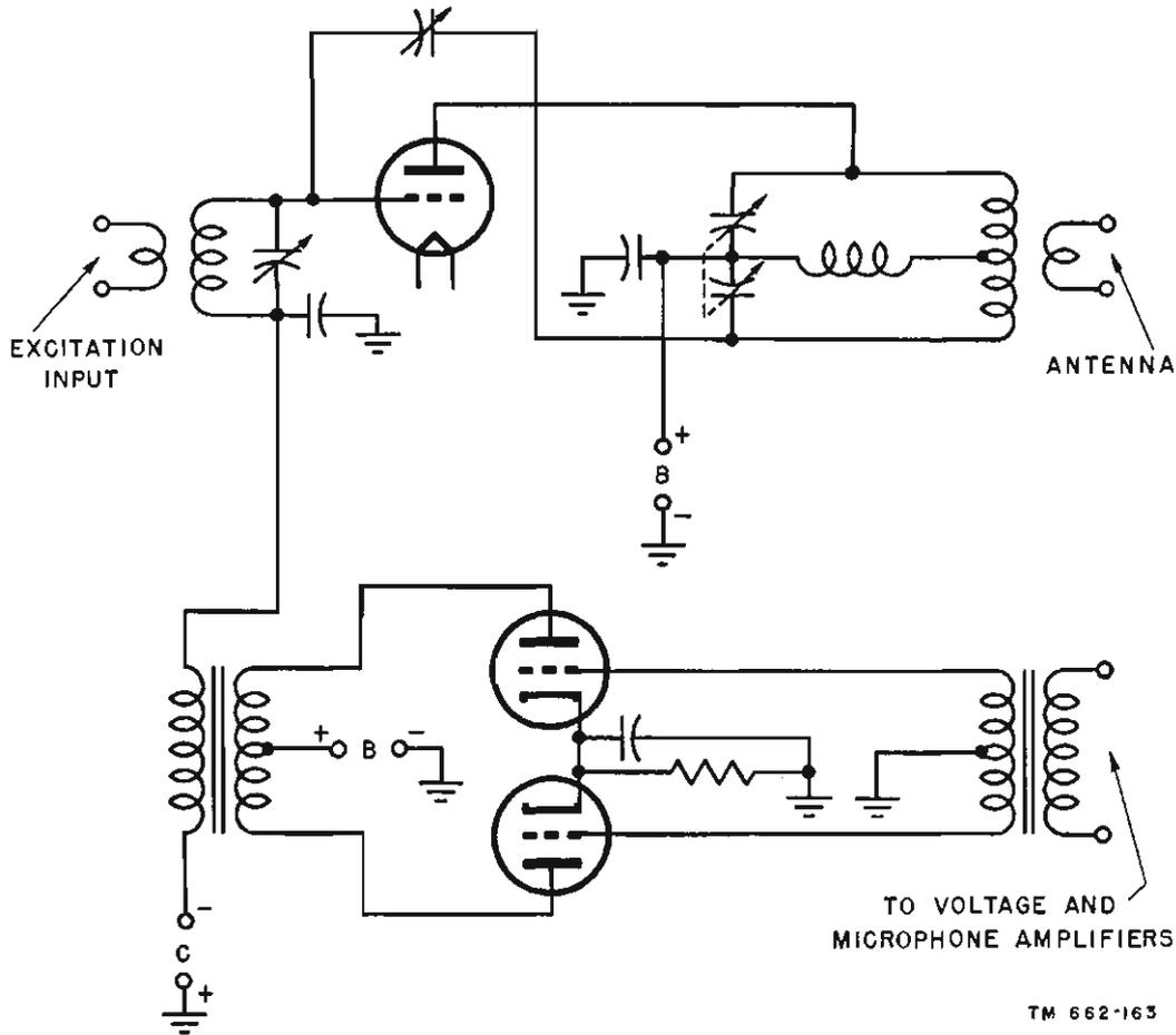
Figure 154. Grid-modulated amplifier.
