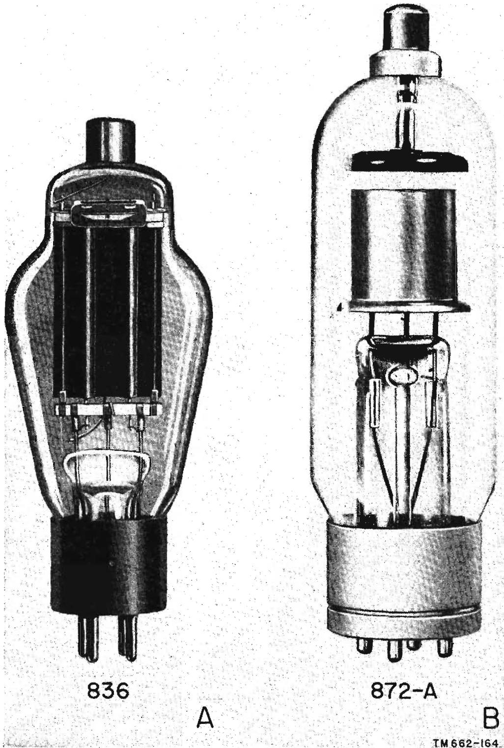
Figure 155. Typical transmitter half-wave rectifiers.
