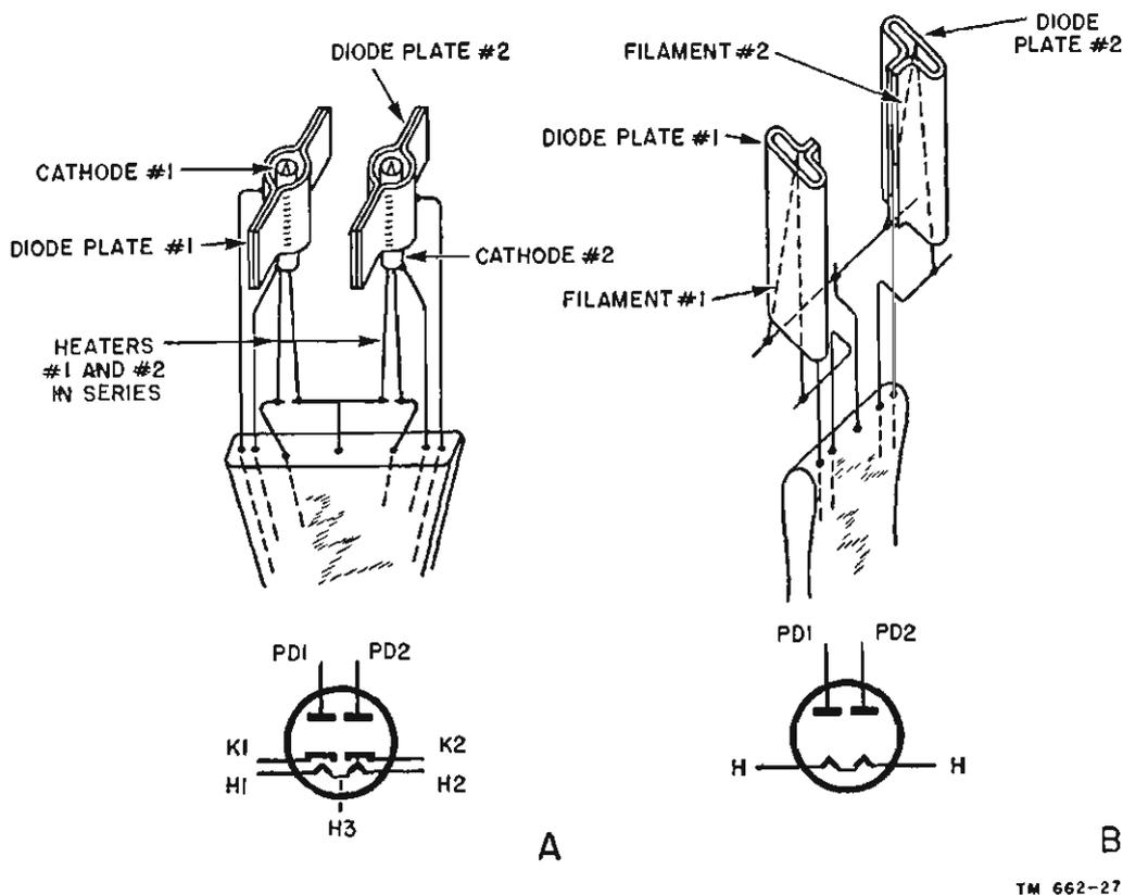
Figure 18. Construction of duo-diode and its schematic representation.
