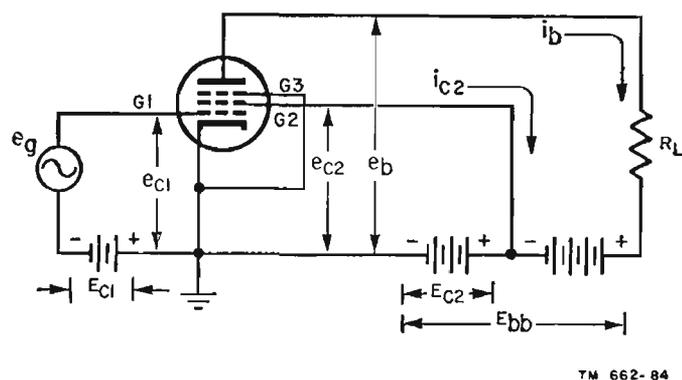
Figure 75. Circuit representation of pentode.
