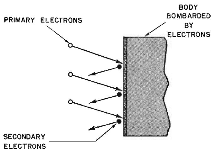
Figure 13. Secondary emission caused by electron bombardment.
