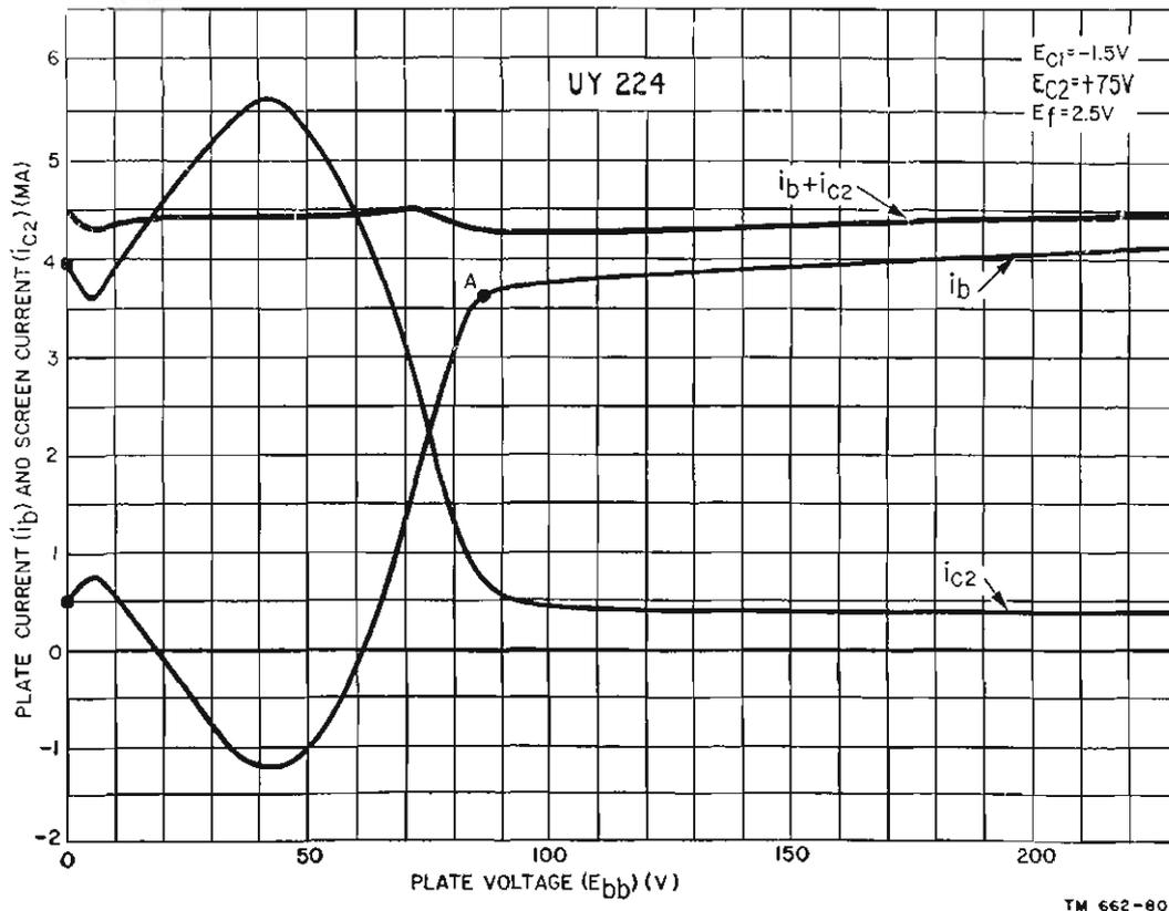
Figure 71. Plate-current plate-voltage characteristic curve for UY-224 tetrode.
