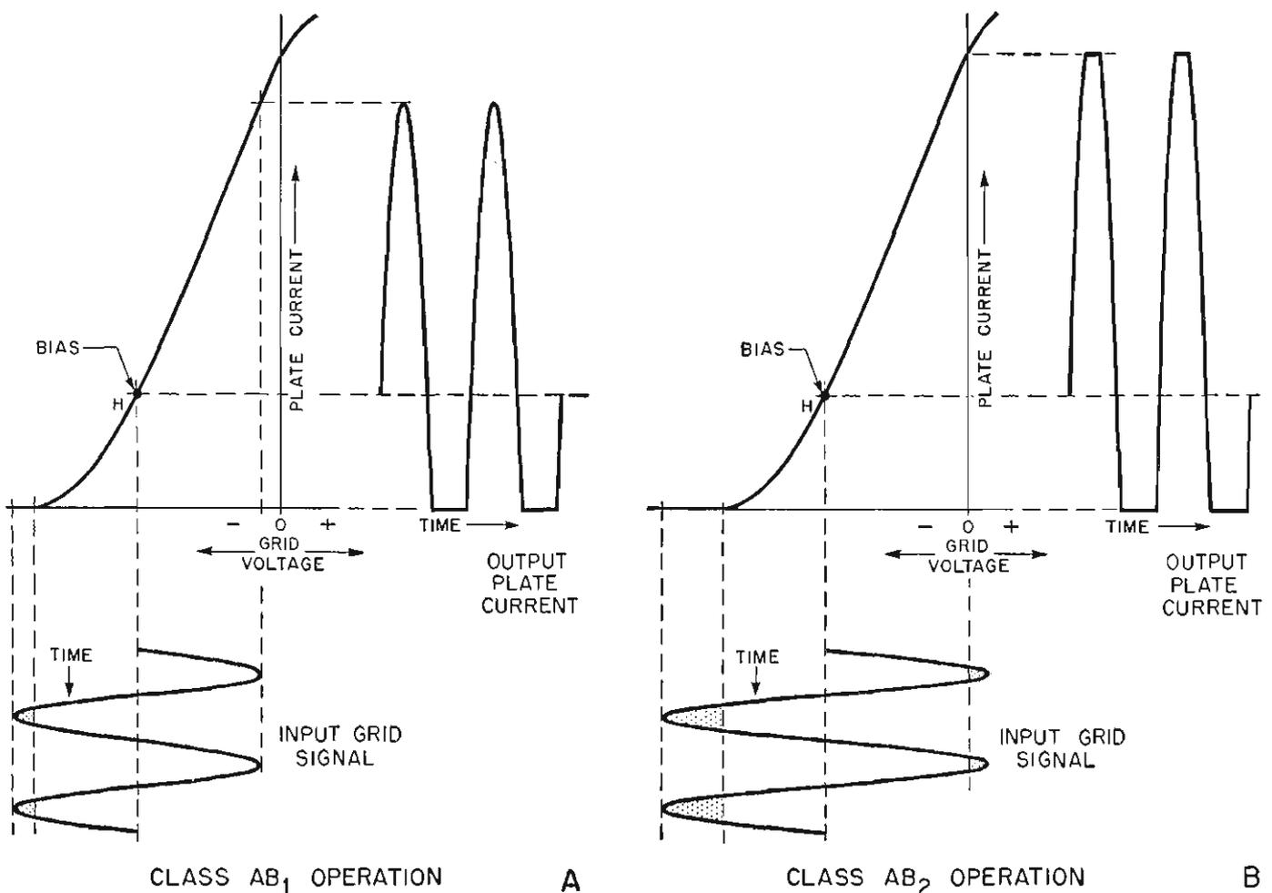
Figure 95. Class AB operation on dynamic characteristic.
