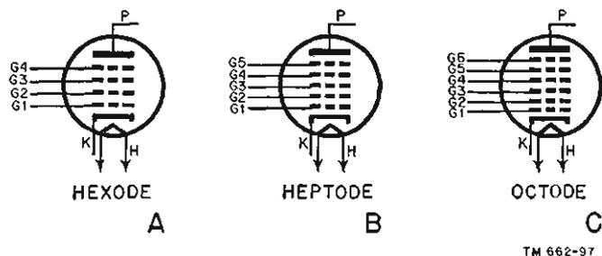
Figure 88. Schematic symbols of multigrid tubes.
