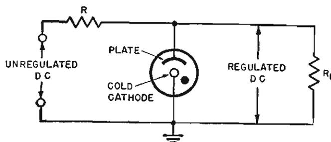
Figure 157. Simple voltage regulator circuit.
