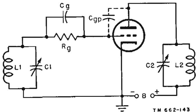
Figure 134. Tuned-plate tuned-grid oscillator.
