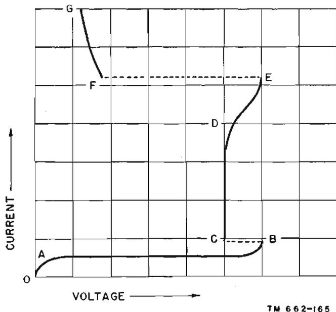
Figure 156. Graphical relations in gaseous conduction.
