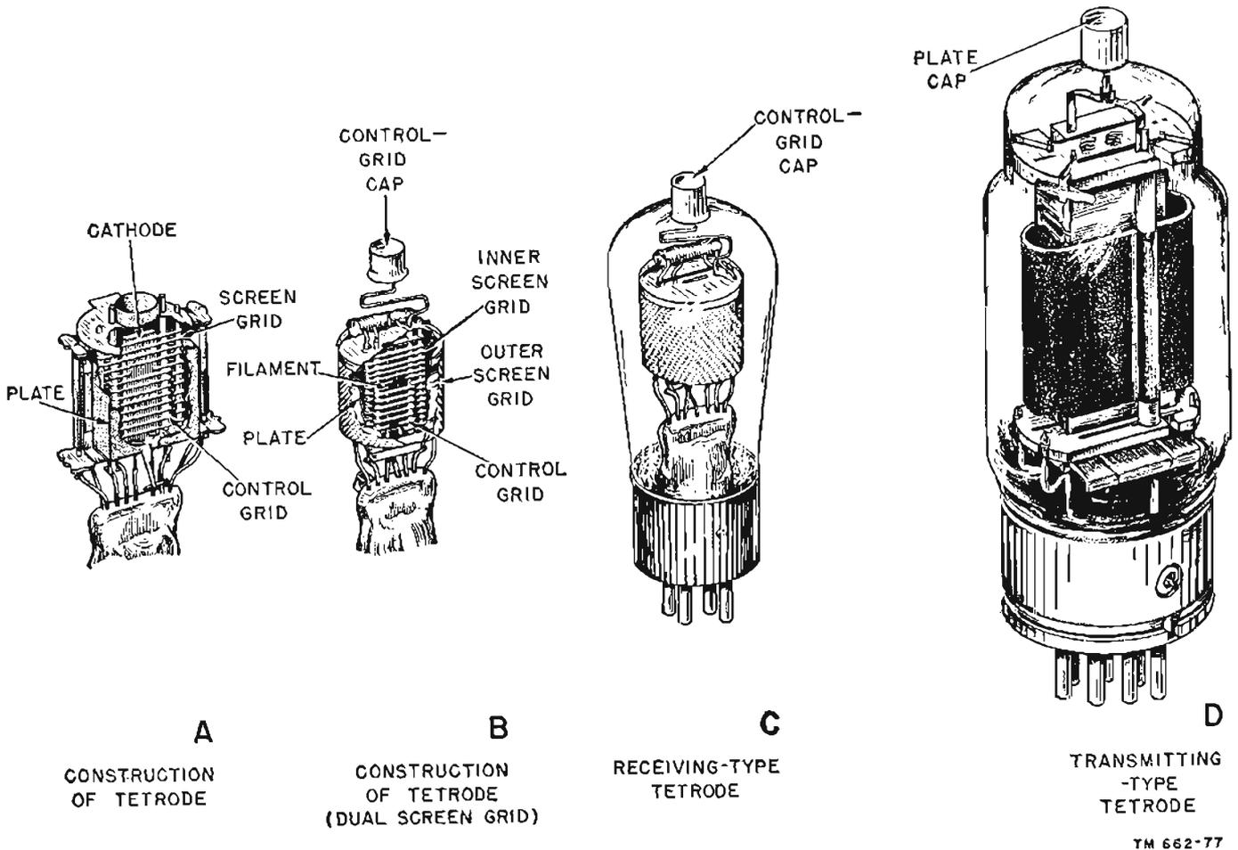
Figure 68. Physical construction of tetrodes.
