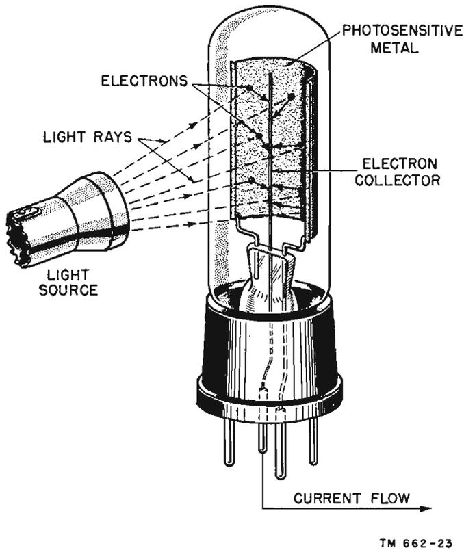
Figure 14. Photoelectric emission of electrons.
