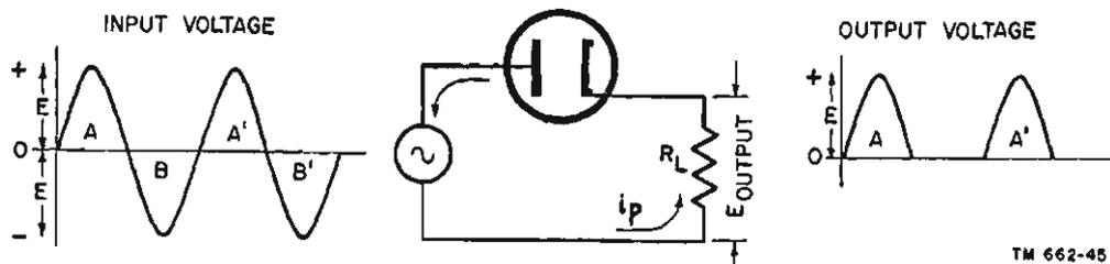
Figure 36. Diagram illustrating unidirectional current flow in diode.
