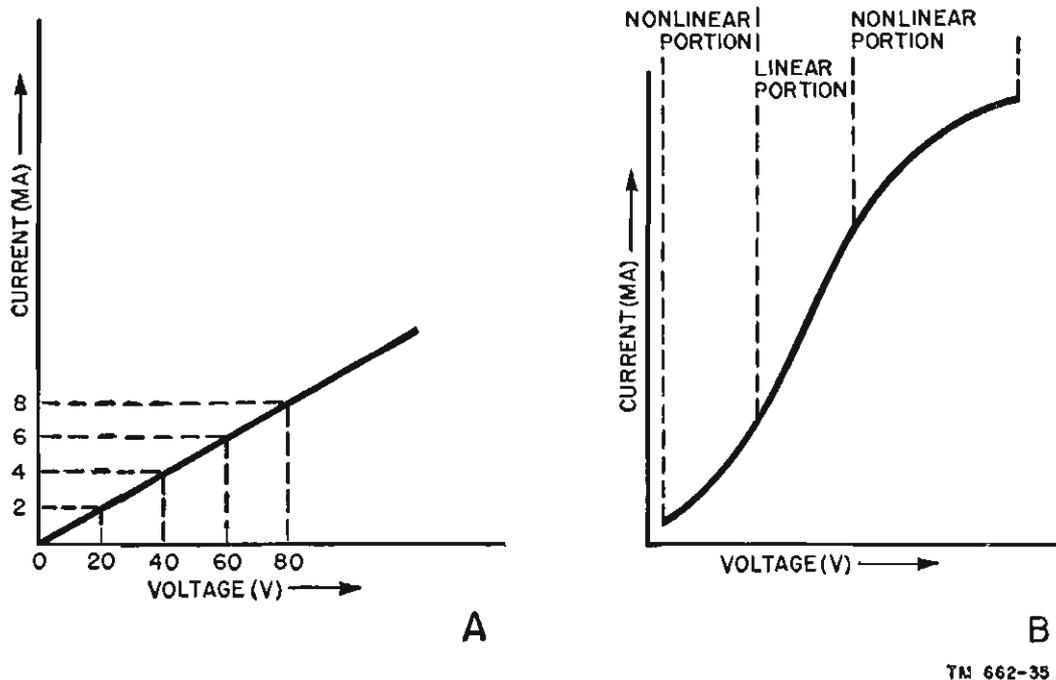
Figure 26. Linear and nonlinear characteristic curves.
