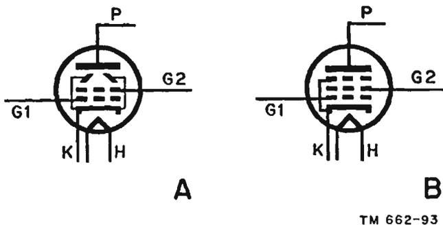
Figure 84. Symbols for beam power tubes.
