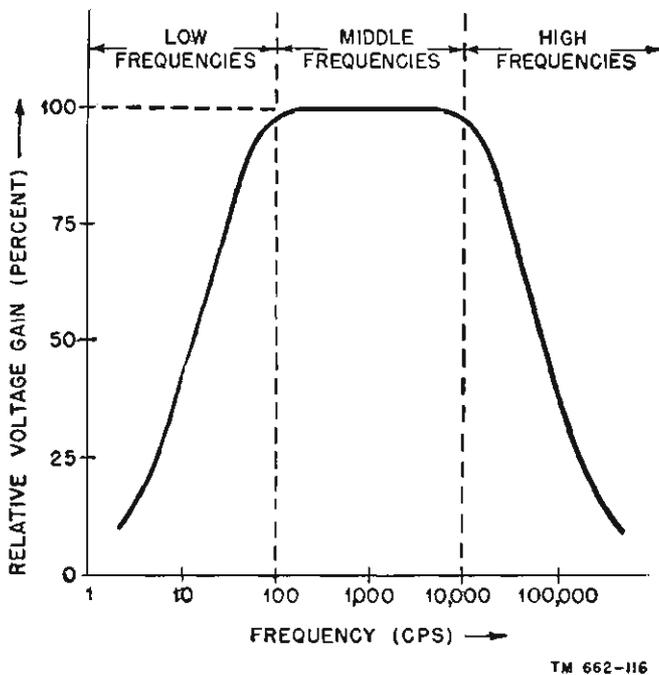
Figure 107. Voltage gain characteristic of typical R-C coupled a-f amplifier.
