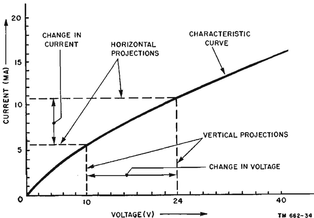
Figure 25. Plot of simple characteristic curve.
