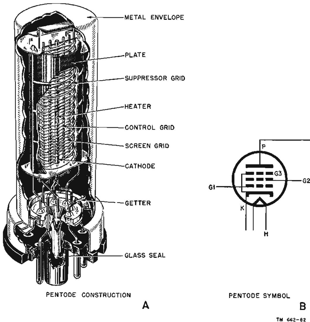
Figure 73. Physical construction (metal-type) and symbol of pentode.
