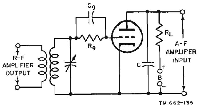
Figure 126. Circuit of grid-leak detector.
