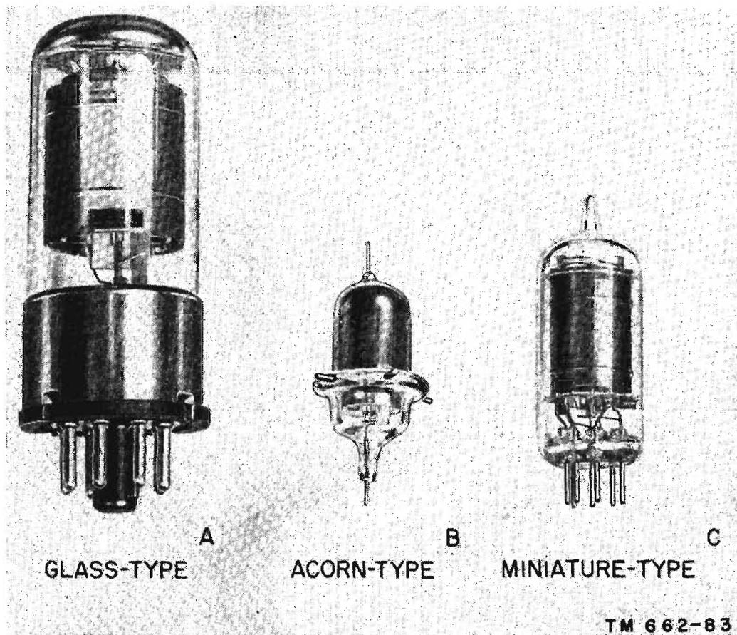
Figure 74. Different types of receiving pentodes.
