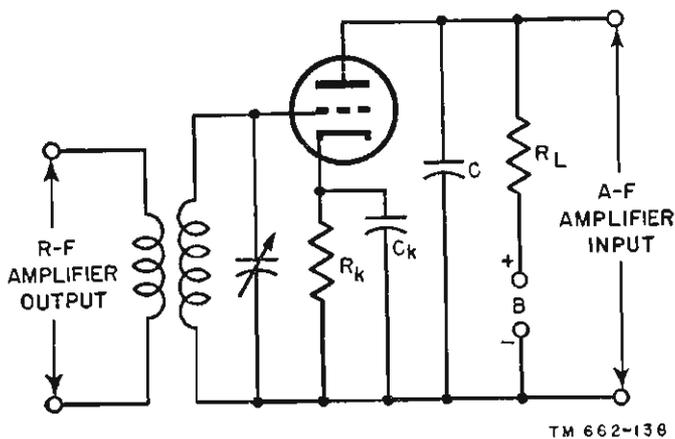
Figure 127. Diagram of plate detector.
