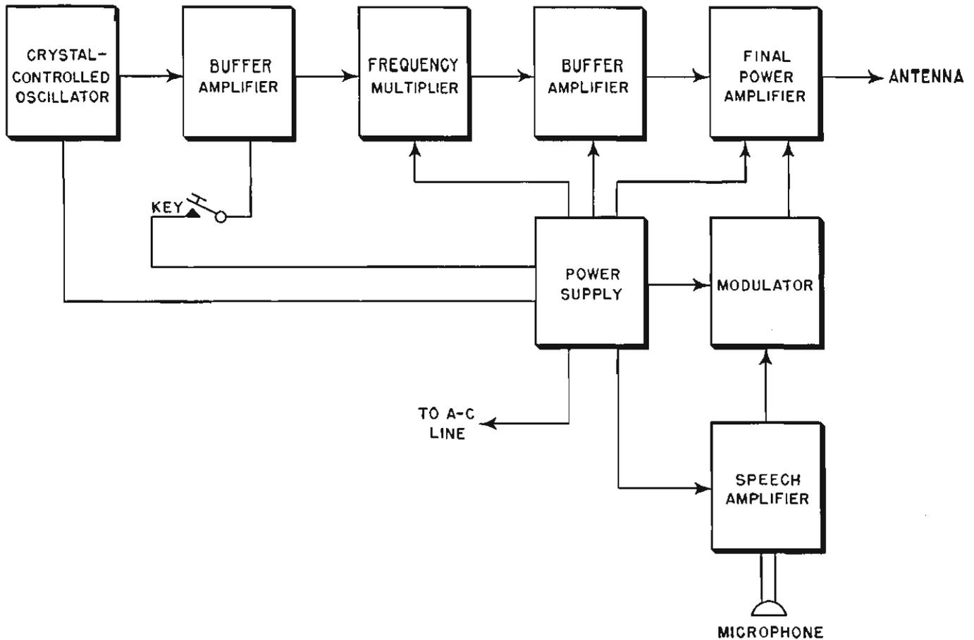
Figure 141. Block diagram of typical transmitter.
