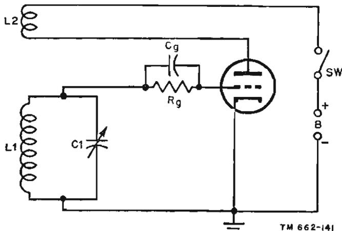
Figure 132. Tuned-grid oscillator.
