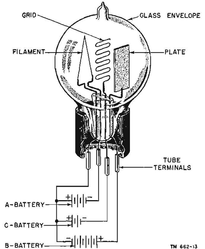
Figure 4. Construction of DeForest's three-element tube, or triode.
