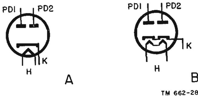
Figure 19. Other schematic representations of duo-diodes.
