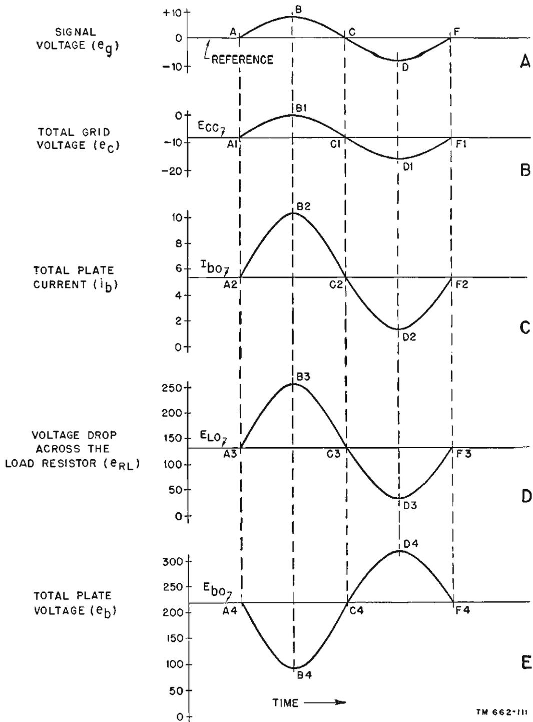
Figure 102. Waveforms in triode amplifier circuit.
