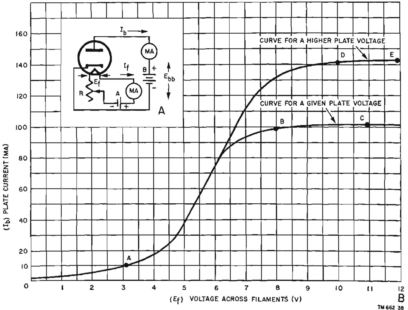
Figure 29. Plate-current filament-voltage characteristic curves.
