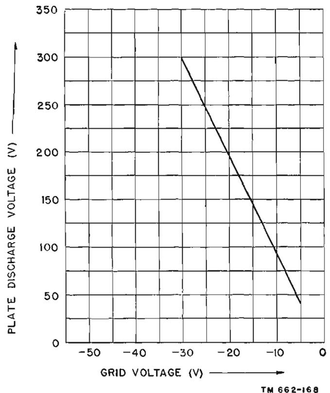
Figure 159. Grid-control characteristic of the 884.
