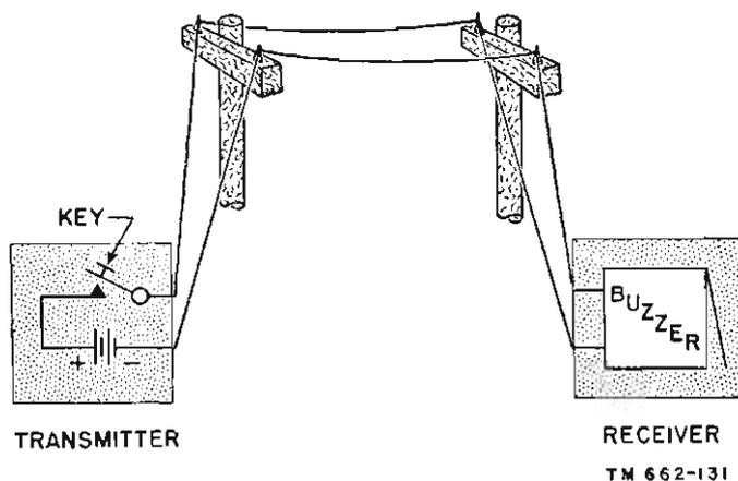
Figure 122. Simple telegraph circuit for communication.
