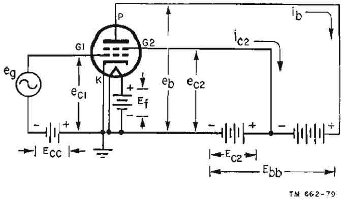
Figure 70. Circuit representation of tetrode.
