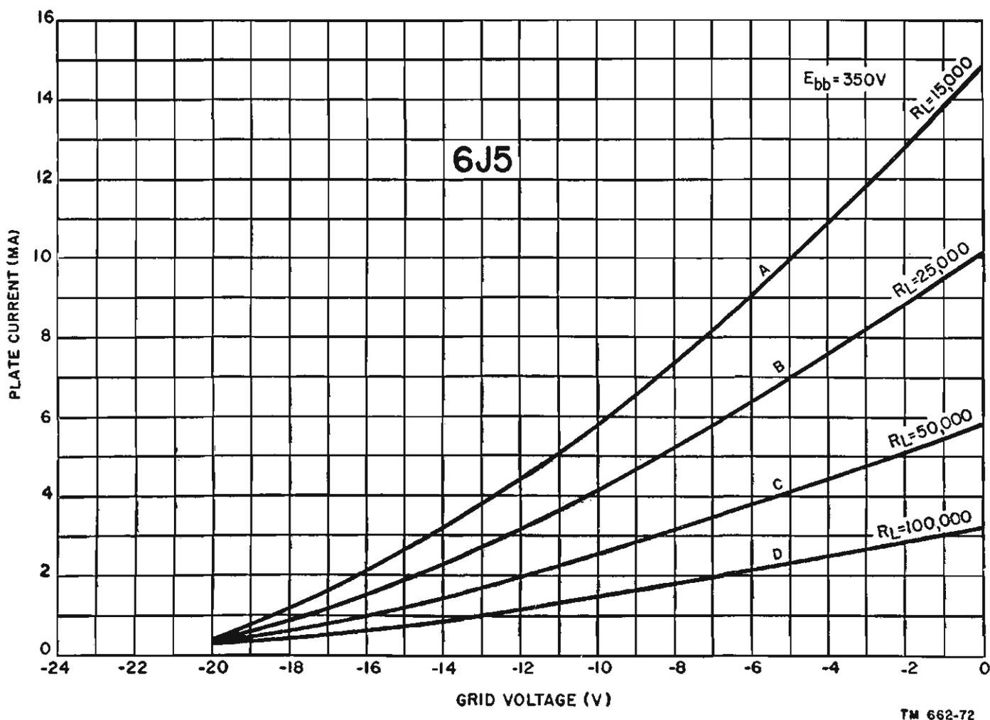
Figure 63. Dynamic transfer characteristic curves for different loads.
