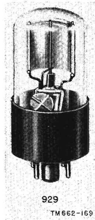
Figure 160. Typical phototube.
