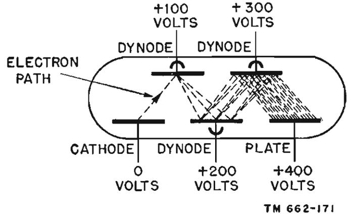
Figure 162. Operation of secondary-emission multiplier.
