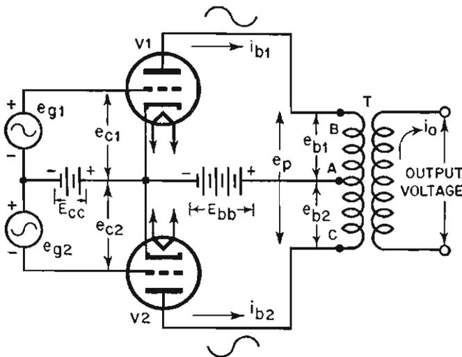
Figure 97. Push-pull triode amplifier circuit.
